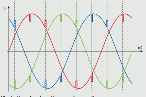
Illustration of undervoltages and overvoltages or "commutation notches"
