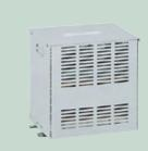
When the sum of the leakage currents of the devices supplied via the part of an installation protected by an RCD is likely to be greater than half the rated residual current ( $I\Delta n$ ) for this RCD, there is a high risk of tripping. This problem can be avoided by using a circuit separation transformer, under TN-S neutral earthing system conditions.
