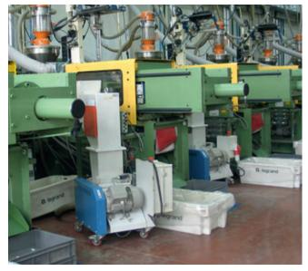
^ In industry, the presence of a large number of motors is the main cause of deterioration of the power factor
