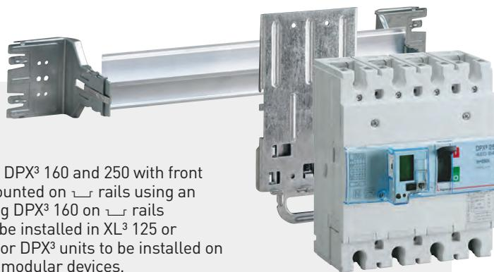
The fixed version DPX<sup>3</sup> 160 and 250 with front terminals are mounted on  $\square$  rails using an adaptor. Mounting DPX<sup>3</sup> 160 on  $\square$  rails enables them to be installed in XL<sup>3</sup> 125 or XL<sup>3</sup> 160 cabinets or DPX<sup>3</sup> units to be installed on the same row as modular devices.
